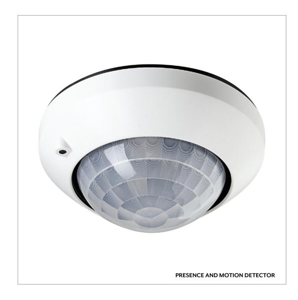
You can rely on the detection characteristics of the motion/ presence detector. When installed at heights of up to six metres, the unit registers everything that is moving within a diameter of approx. 20 m. For this, the device has three PIR sensors operating independently of each other. All settings are made conveniently using the Clever Config app.
