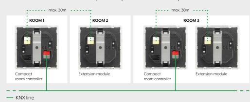
The push-button extension module complements an F 50 installation with additional, cost-effective satellites.
